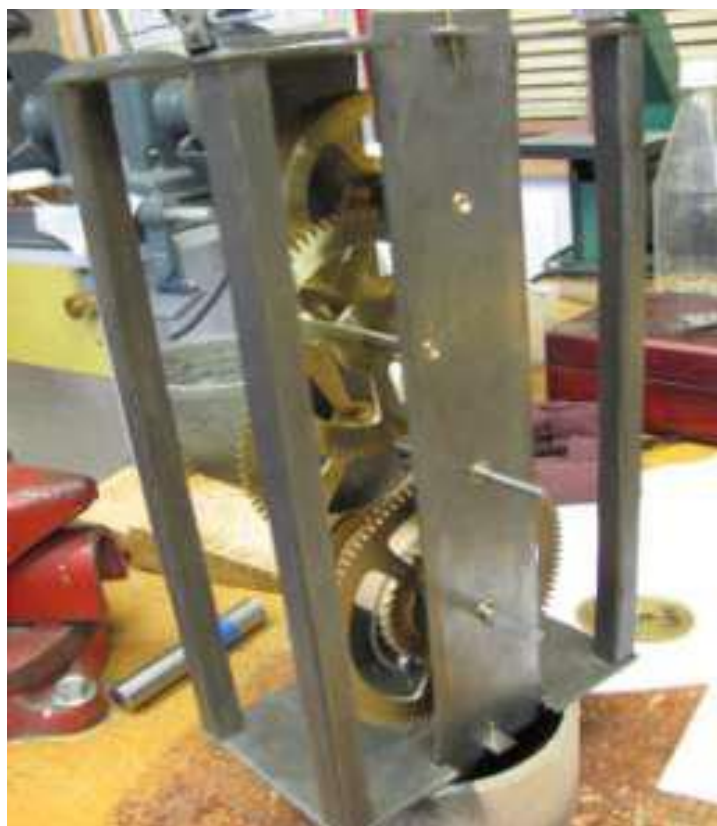
Figure 15. First assembly of wheel train between plates.
