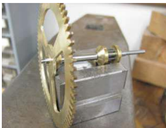
Figure 13. Wheels and pinions staked to arbors.
