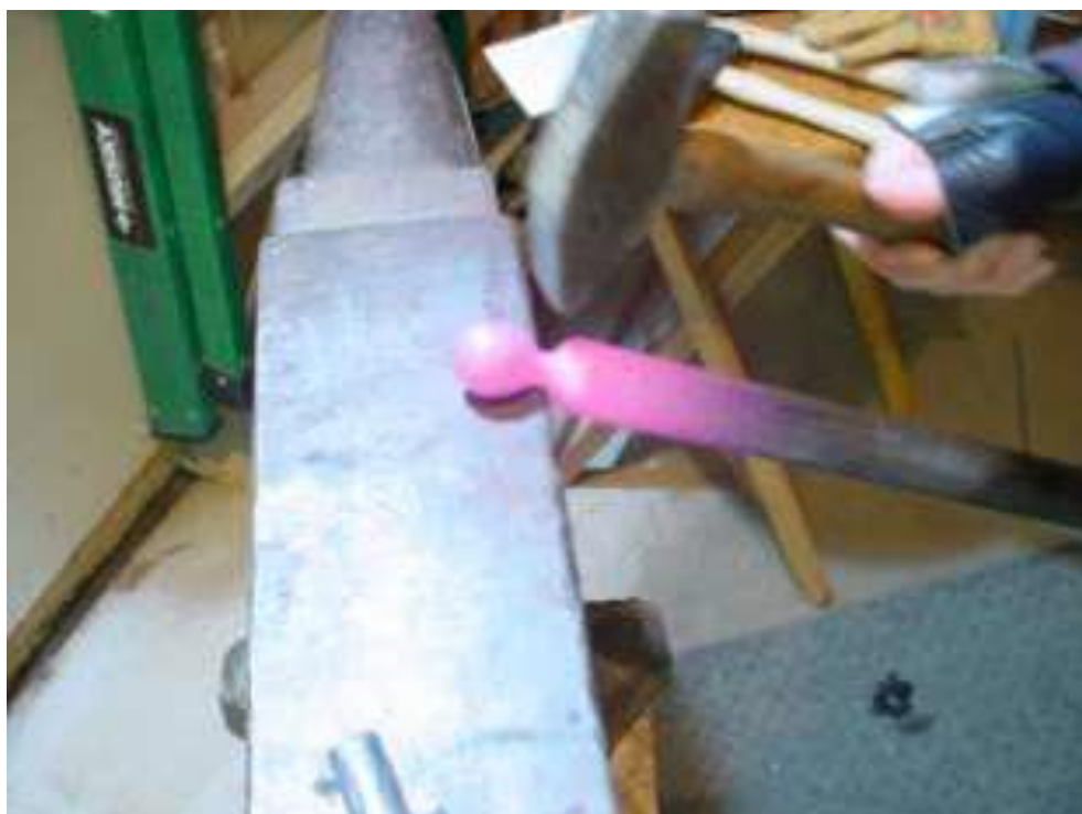
Figure 3. Forging the flower bulbs using blacksmith tools.
