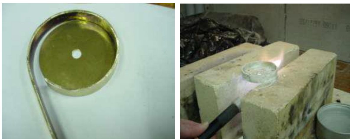
Figure 6. The crown wheel is fabricated from two pieces of brass soldered together.
