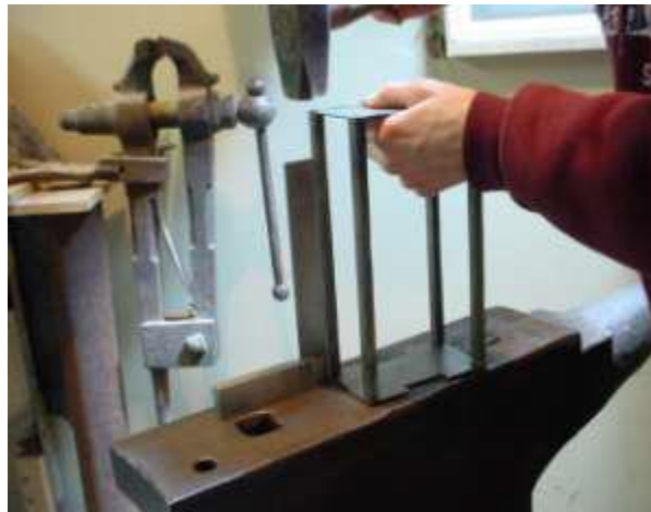
Figure 10. Forging and assembling clock frame.
