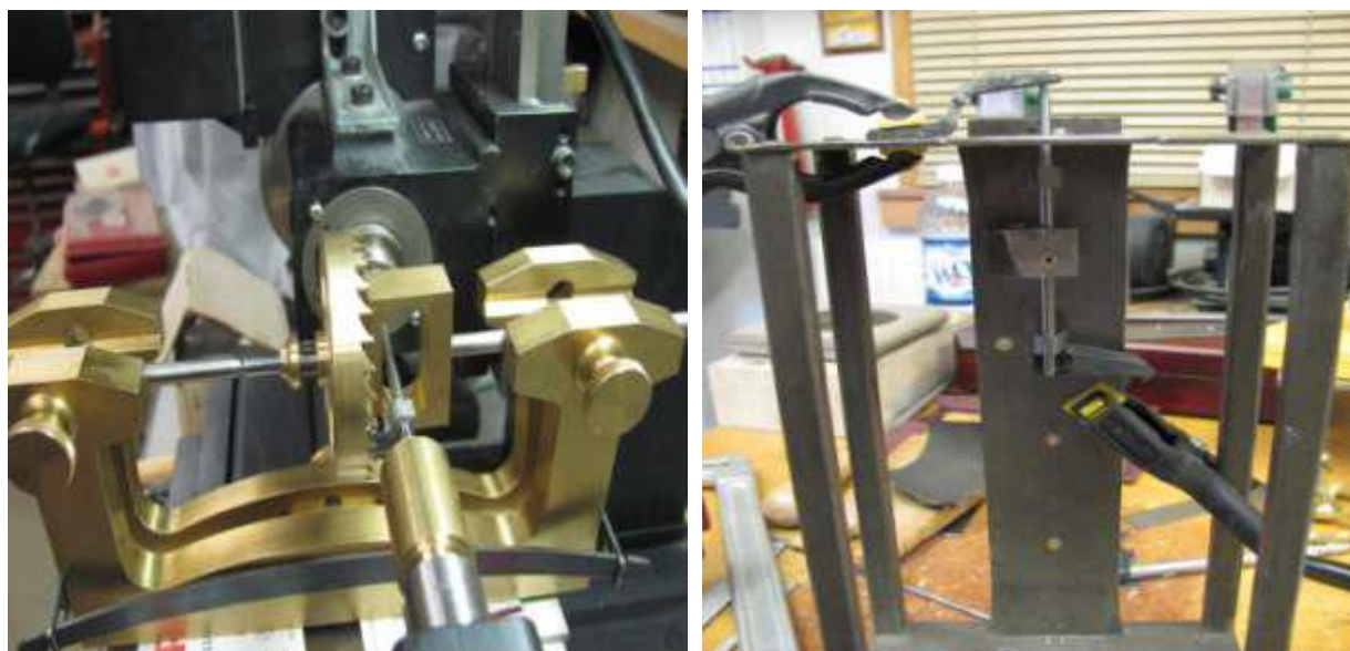
Figure 16. Depthing of crown wheel and testing escape pallet bridges.
